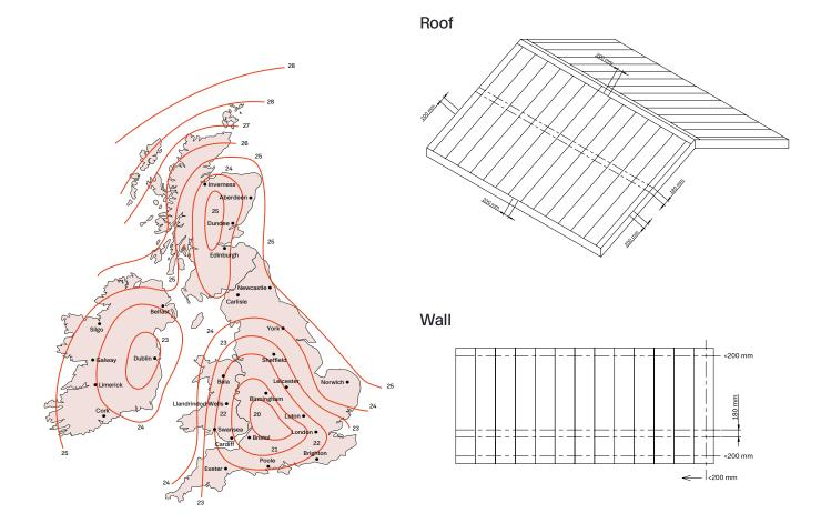
When building over 3 stories or in exposed locations the structural engineer should complete a wind uplift calculation and provide Catnic Urban with the details so the best fixing solution can be developed.
